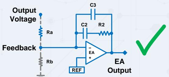
$$H_c(s) = \frac{\omega_{P0}}{s} \frac{\left(\frac{s}{\omega_{Z1}} + 1\right)}{\left(\frac{s}{\omega_{P1}} + 1\right)}$$
