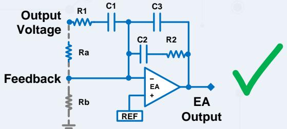
$$H_c(s) = \frac{\omega_{P0}}{s} \frac{\left(\frac{s}{\omega_{Z1}} + 1\right)\left(\frac{s}{\omega_{Z2}} + 1\right)}{\left(\frac{s}{\omega_{P1}} + 1\right)\left(\frac{s}{\omega_{P2}} + 1\right)}$$
