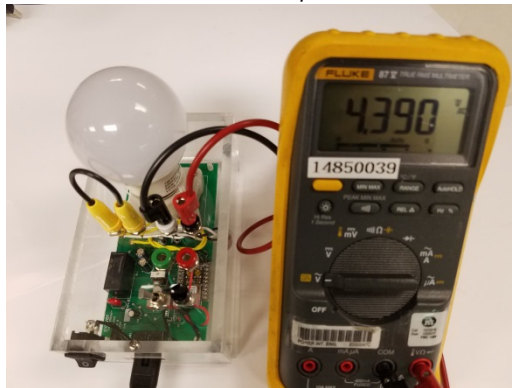
Figure 14 – Leakage Voltage, Bulb is OFF.
