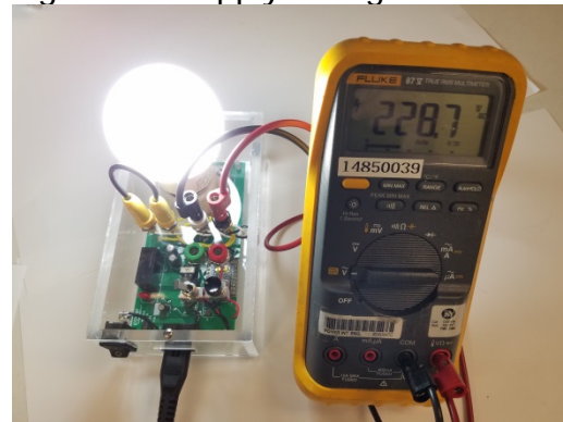
Figure 15 – Input Voltage, Bulb is ON.
