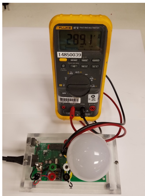
Figure 12 – Input Current, With BLE Load, 230 VAC.
