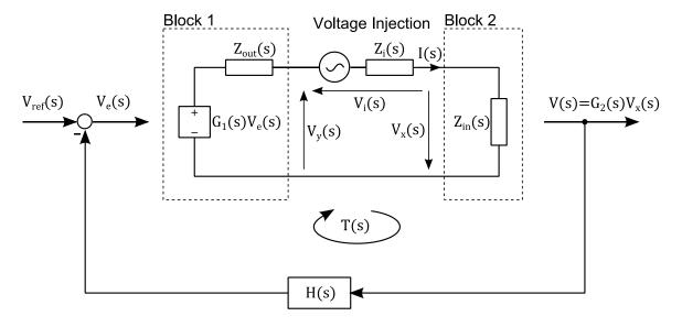
The injecting source is modeled with a voltage source and a series impedance  $Z_i(s)$ .
