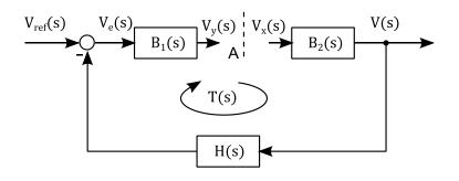
The measured loop gain then equals  $T_m(s) = \frac{V_y(s)}{V_x(s)}$ .
