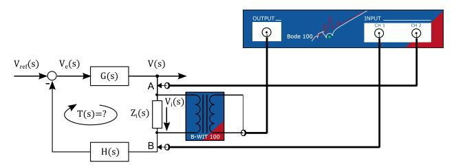
The analyzers inputs are connected on both sides of the injection resistor using coaxial cables or voltage probes. The loop gain is then measured by measuring the complex voltage gain from point A to B.
