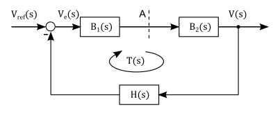
Applying a test voltage  $V_x(s)$  after the injection point A leads to the response voltage  $V_y(s)$  before the injection point.
