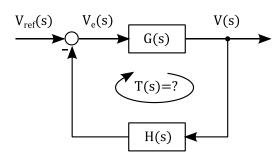
The output signal or voltage V(s) follows the reference voltage  $V_{ref}(s)$  by the relation
