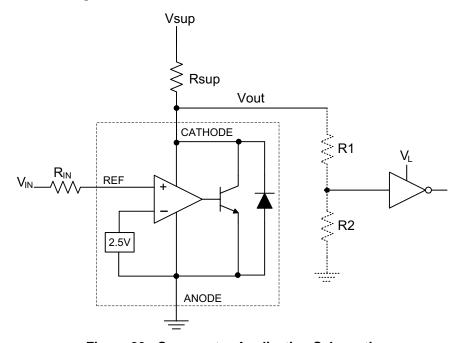
Figure 20. Comparator Application Schematic
