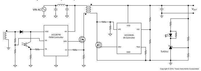
Figure 25. Isolated Flyback with Optocoupler
