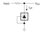
Figure 16. Test Circuit for Ioff
