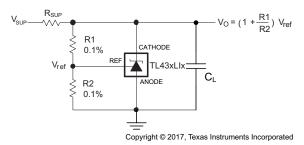
Figure 23. Shunt Regulator Schematic
