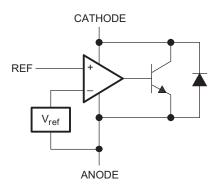
Figure 18. Equivalent Schematic
