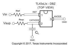
Figure 38. DBZ Layout example
