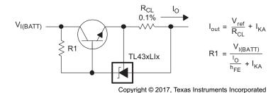
Figure 36. Precision Current Limiter
