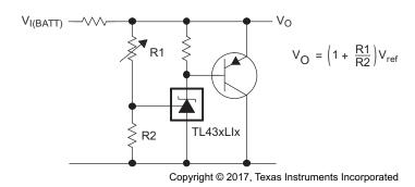
Figure 29. High-Current Shunt Regulator
