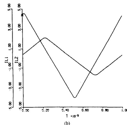
Fig. 5. Simulated waveforms for (a)  $V_M$  and  $V_S$  for  $R_0 = 7.5 \Omega$ ,  $I_a = 2.25$  A,  $V_0 = 16.8$  V,  $t_2 = 200$  nS, (b)  $i_{L1}$  and  $i_{L2}$  for the same conditions.
