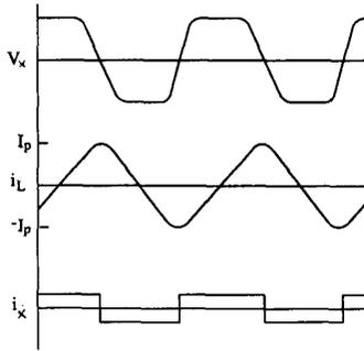
Fig. 2. Relevant waveforms for resonant pole circuit.
