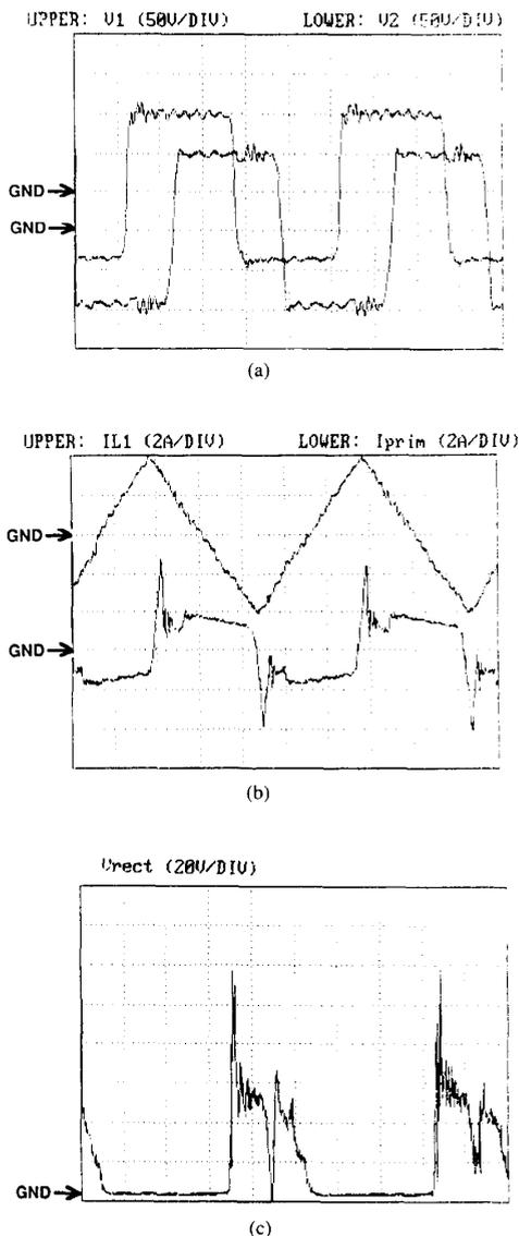
Fig. 9. Experimental oscillograms of converter operation. (a)  $V_M$  and  $V_S$  for 99.2-W-load,  $I_0 = 6.4$  A,  $V_0 = 15.5$  V, time scale = 200 nS/div. (b)  $I_{L1}$  and  $I_{prim}$  from same conditions. (c)  $V_{rect}$  from same conditions.
