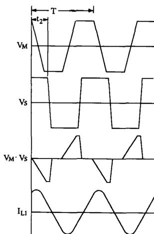
Fig. 4. Relevant waveforms for pseudo-resonant dc/dc converter.
