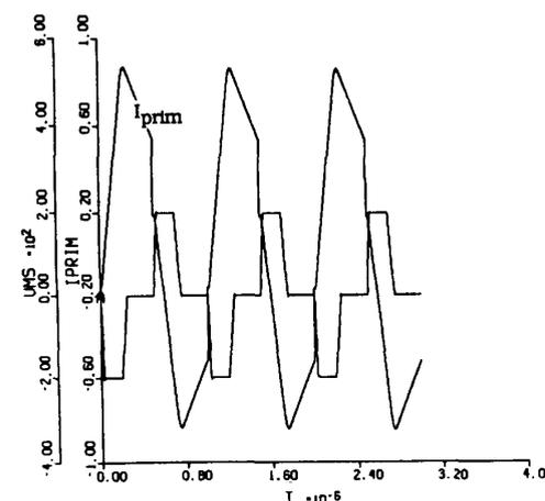
Fig. 6. Simulated waveforms showing transformer primary voltage  $V_{MS}$  and primary current  $I_{\text{prim}}$ . Same conditions as Fig. 5.
