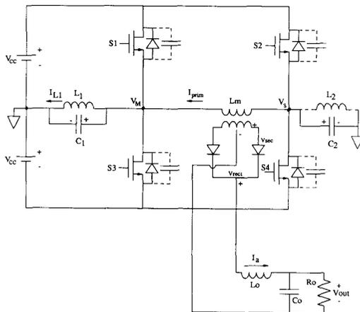
Fig. 3. Proposed pseudo-resonant dc/dc converter.
