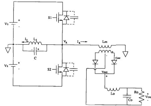
Fig. 1. Resonant pole circuit schematic.
