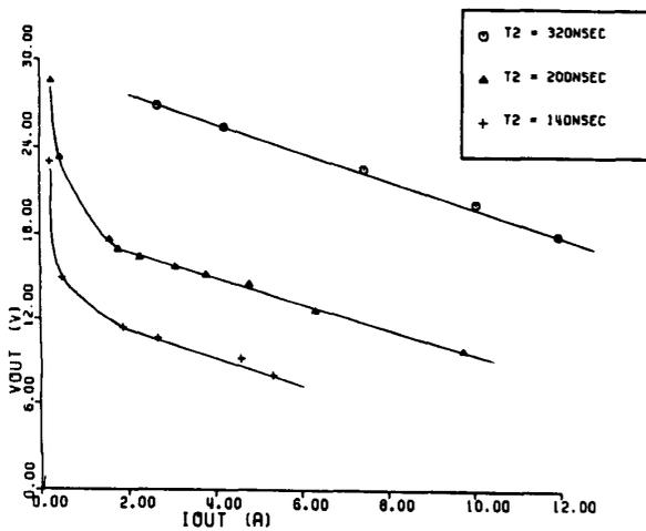
Fig. 8. The output  $V_0$ - $I_0$  characteristics of the pseudo-resonant converter obtained through simulation.
