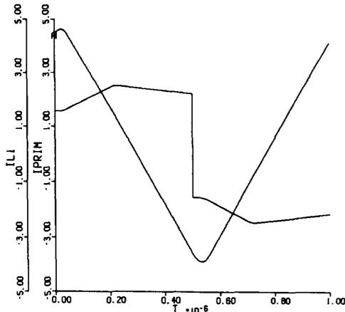
Fig. 7. Simulated waveforms showing  $I_{prim}$  and  $I_{L1}$  for  $R_0 = 1 \Omega$ ,  $I_{in} = 9.6$  A,  $V_0 = 9.6$  V,  $t_2 = 200$  nS.
