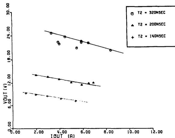
Fig. 10. Experimentally obtained  $V_0$ - $I_0$  plane from the pseudo-resonant converter.
